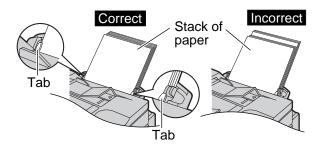
Adjust the width of the guides to the size of the recording paper by sliding the right side of the guides.
